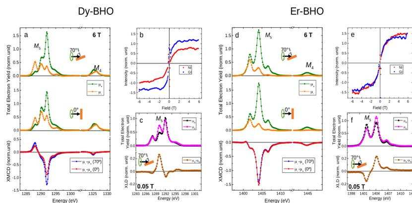
Fig. 1. a)-d) XAS and XMCD of Dy- and Er- BHO metallocenes; b)-e) Magnetic intensity versus external magnetic field in Dy-HBO and Er-BHO; c)-f) XLD for Dy- BHO and Er- BHO.
