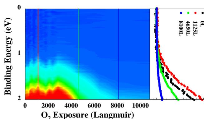
Fig. 1 Electrical property change of InSe according to oxidation progress. Scheme of the valence band structure base on the Fermi level ( $E_F$ , 0eV) as a contour map
